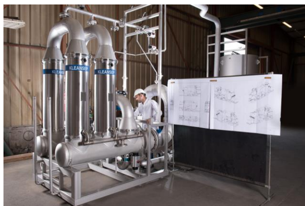
Industrial equipment and process engineering: filtration skid
